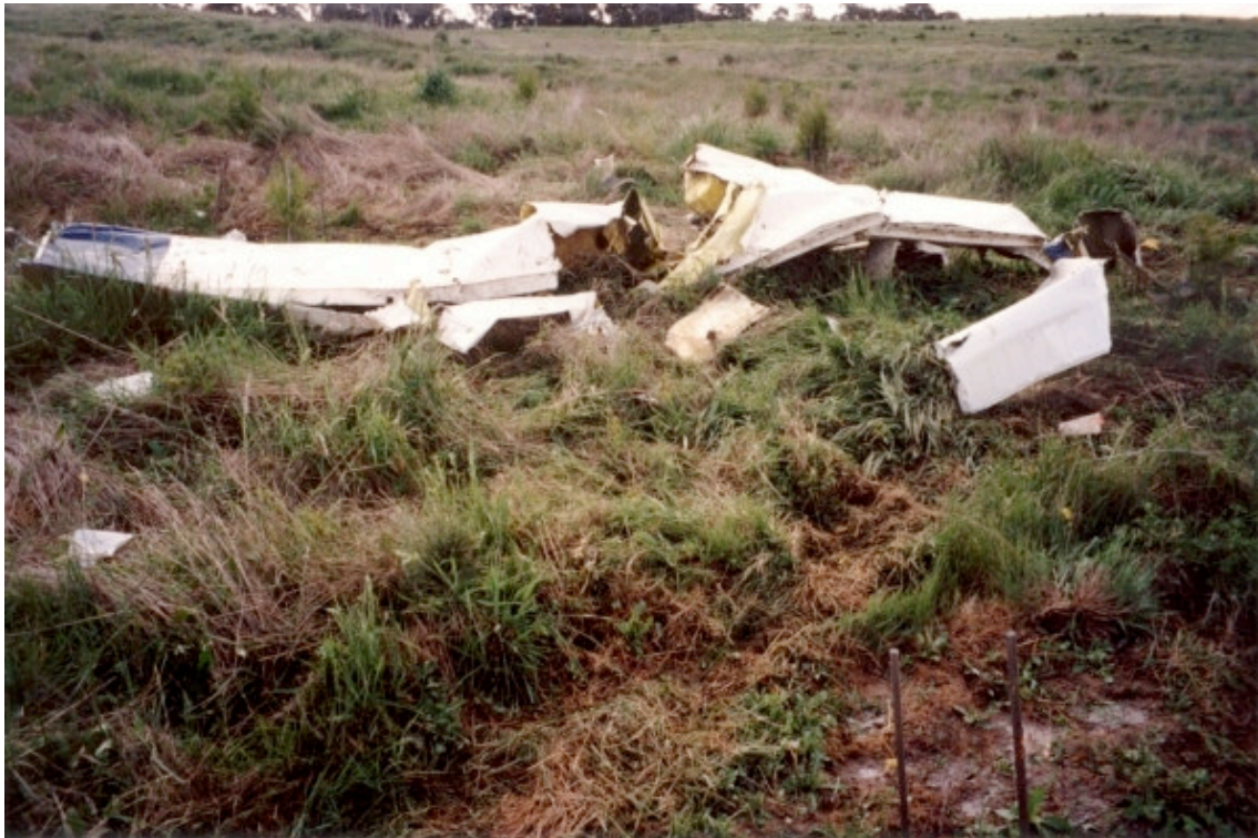
Figure 8. Wreckage of a light aircraft VFR into IMC accident
