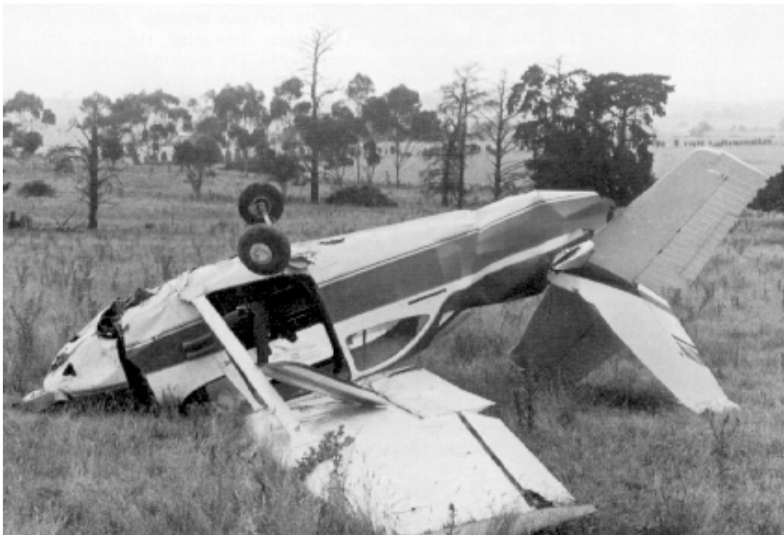
Figure 2. An aircraft substantially damaged as a result of a precautionary landing 2
