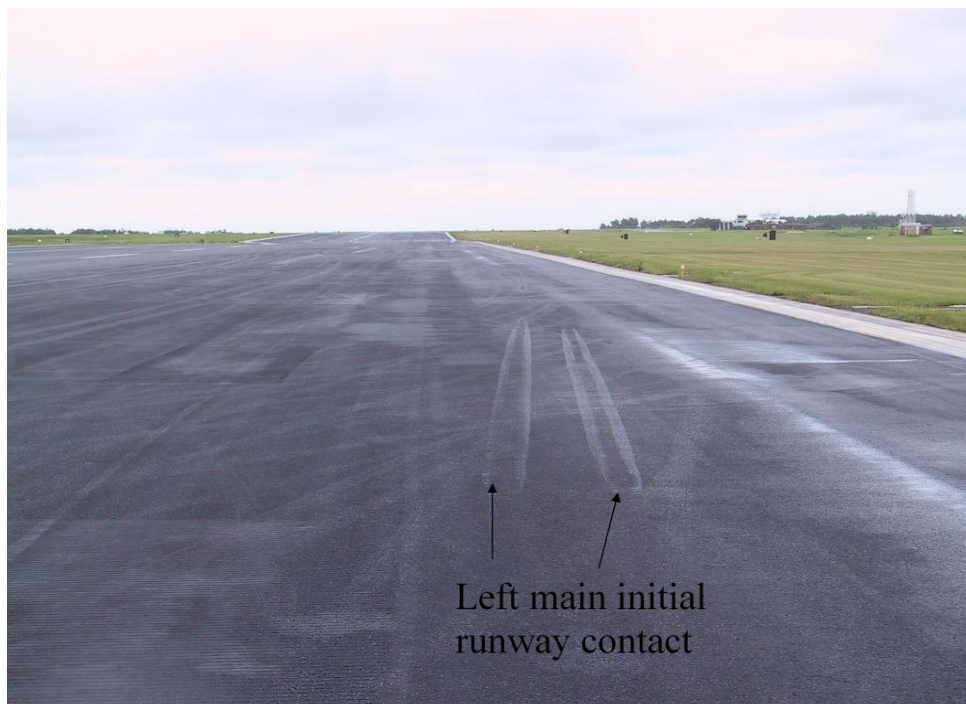
Figure 7: Lateral touchdown position of the left main landing gear
